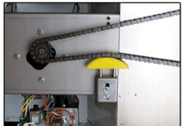
Automatic drive chain tensioner maintains proper tension on the chain at all times.
