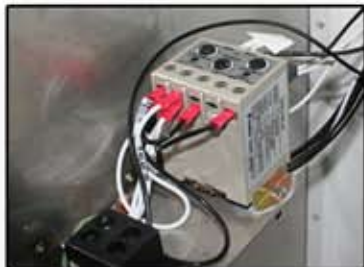
The shock relay safety switch instantly turns off the motor if anything jams the drive system.
